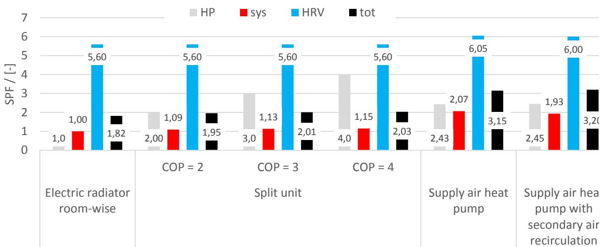
Fig. 11 Annual (heating season) SPFs of the heat pump (“HP”), heating system (“sys”), HRV and total HVAC (“tot”), according to equations (1)-(4)
