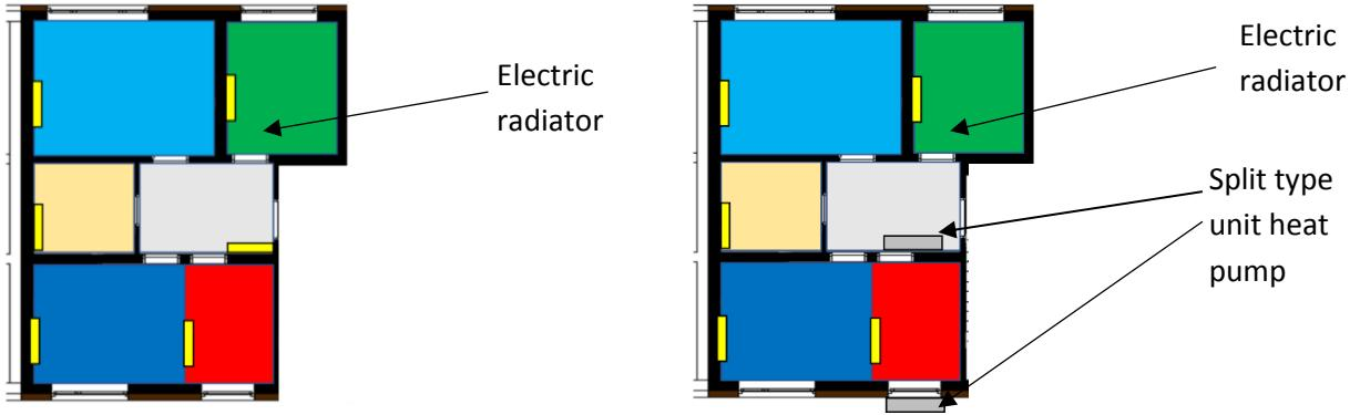
Fig. 8: 2D view of the flat with (left) electric radiators and (right) the HP split unit with recirculation of air in the corridor (Ochs et al. 2017). The indoor unit is installed in the corridor, while the outdoor unit can be integrated in the façade. All the rooms (except the corridor) are equipped with electric radiators
