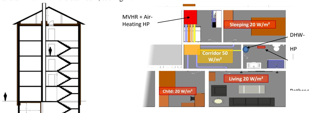
Fig. 1: (left) Typical MFH and (right) heat load (in  $\text{W}/\text{m}^2$ ) of the thermal zones with optional recirculation air heating in the corridor; Ventilation and HP in the kitchen and DHW HP in the corridor
