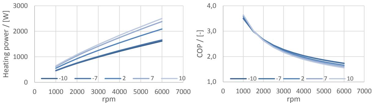
Fig. 6: Performance map of the thermal power of the heat pump (left) and the COP (right) depending on the rpm of compressor and ambient air temperature [°C] – Supply air heat pump system
