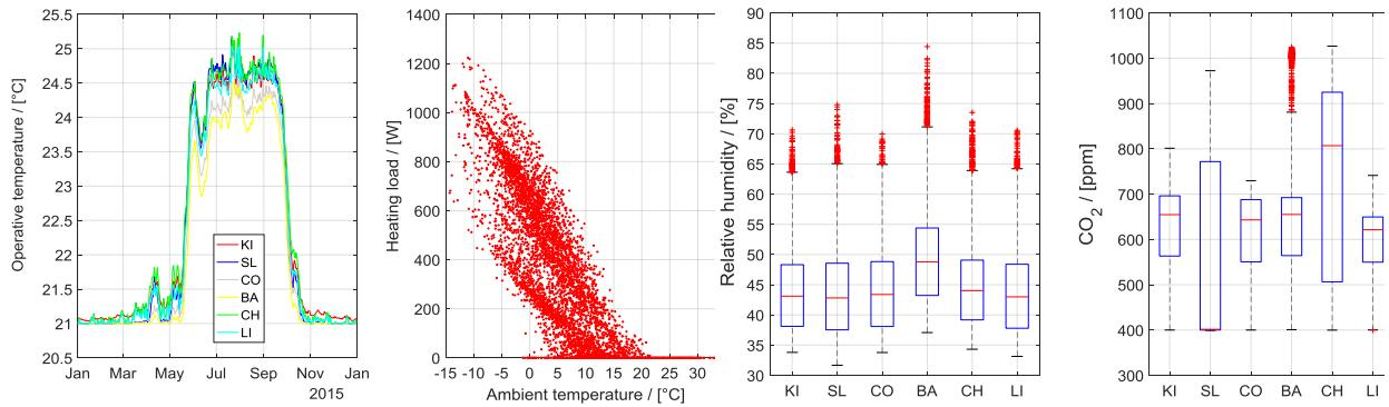
Fig. 9: Electric radiator room-wise system - daily average operative temperatures for each room of the flat (left) and hourly heating load versus ambient temperature (2nd from left); KI: Kitchen, SL: Sleeping Room, CO: Corridor; BA: Batch room; CH: child room, LI: Living room; Box plot of relative humidity (2nd from right) and CO<sub>2</sub> concentration (right) for each room of the flat; CO<sub>2</sub> ambient concentration is 400 ppm
