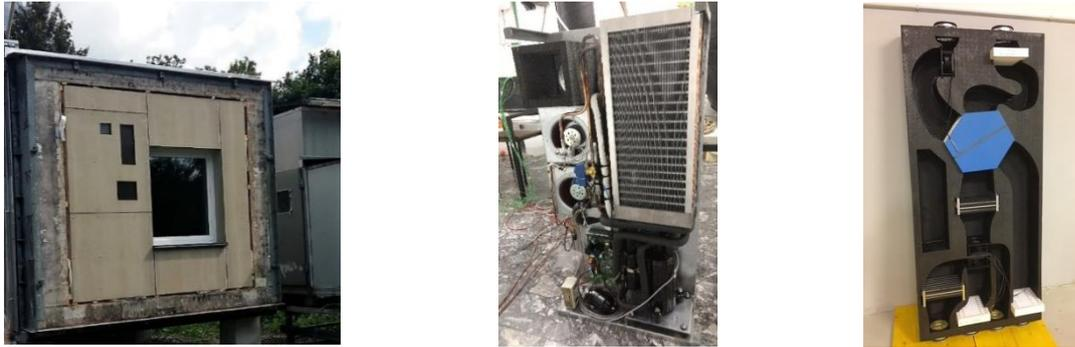
Fig. 5: Outside view of the outdoor unit integrated into the prefabricated timber frame façade in the Passys test cell (left), outdoor unit in the laboratory at the UIBK (center) and indoor unit
