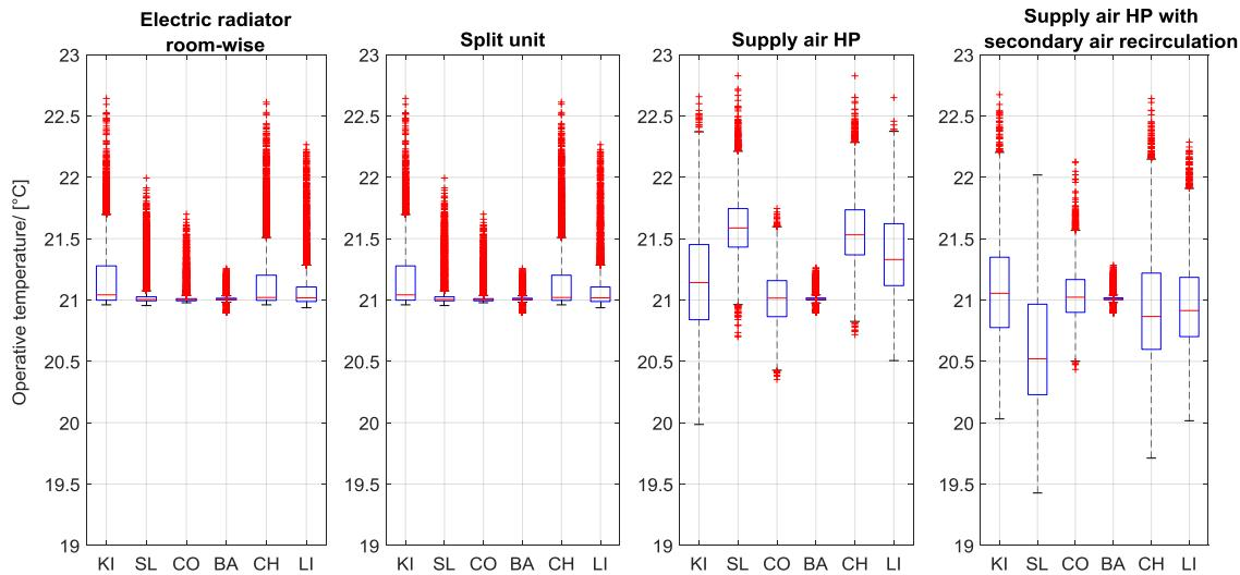
Fig. 10: Box plot of operative temperatures (hourly average) during the heating season for the four heating concepts
