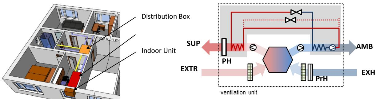
Fig. 2: 3D view of the flat with the supply air heat pump system (left) and scheme of the heat pump in combination with MVHR (right). "PH" and "PrH" represent the post-heater and the pre-heater, respectively
