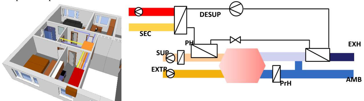
Fig. 3: 3D view of the flat with the supply air heat pump system with recirculation air in the corridor (left) and refrigerant cycle scheme (right). "PH" and "PrH" represent the post-heater and the pre-heater, respectively. "DESUP" indicates the de-superheater that is used to heat the recirculation air in the corridor, (Siegele 2018)
