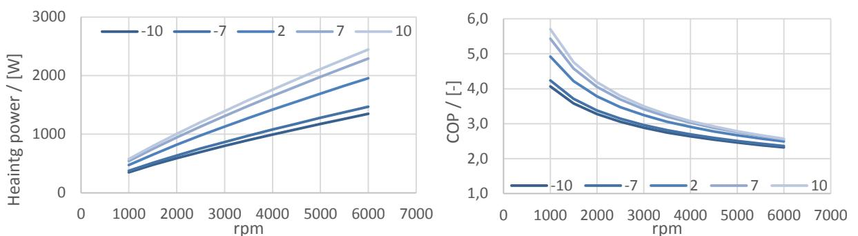
Fig. 7: Performance map of the total thermal power of the heat pump (left) and the COP (right) depending on the rpm of compressor and ambient air temperature [°C] – Supply air heat pump with secondary air recirculation system. Additional ambient air of 200 m<sup>3</sup>/h was used as source. The total heating power was split between the condenser (50%) for the supply air and the de-superheater (50%) for secondary air.
